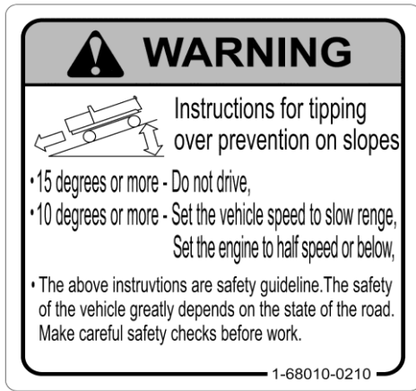
(13) Precautions when travelling downhill (1-68010-0210)
